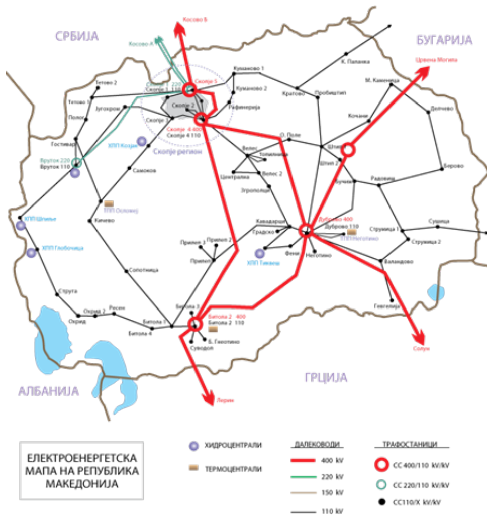
Figure 6. High voltage transmission grid in Macedonia (Electricity map of the Republic of Macedonia, Source: AD MEPSO, http://www.mepso.com.mk/Details.aspx?categoryID=114 )
