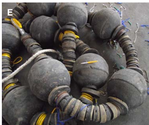
Plate 1. Photographs showing examples of ground gear used currently or historically in the South African Hake Trawl fishery. Photograph (a) and (b) depict an inshore ground rig with small (less than 250 mm) rubber discs and small (100 mm) rubber spacers. Large heavy steel bobbins and large rubber rockhopper disks are shown in photograph (c) which was taken aboard a foreign vessel fishing on the inshore grounds of the Agulhas Bank in the 1980's. Current offshore ground rigs with rockhopper disks (d) and solid rubber bobbins (E) are also shown. Larger steel bobbins (610 mm maximum diameter) which are used on some vessels in offshore grounds are also depicted (F). These steel bobbins are no longer frequently deployed in this fishery but are within the size restrictions of current permit conditions. Some photos courtesy of Rob Whitehead.
