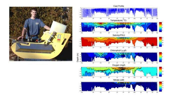
The Mariner Shuttle undulating oceanographic sampling system (left) carries sensors for temperature, salinity, chlorophyll, oxygen and nitrate. Payload output (right) of depth, temperature, salinity, chlorophyll, oxygen, and nitrate. The Shuttle also carries a continuous plankton recorder mechanism.
