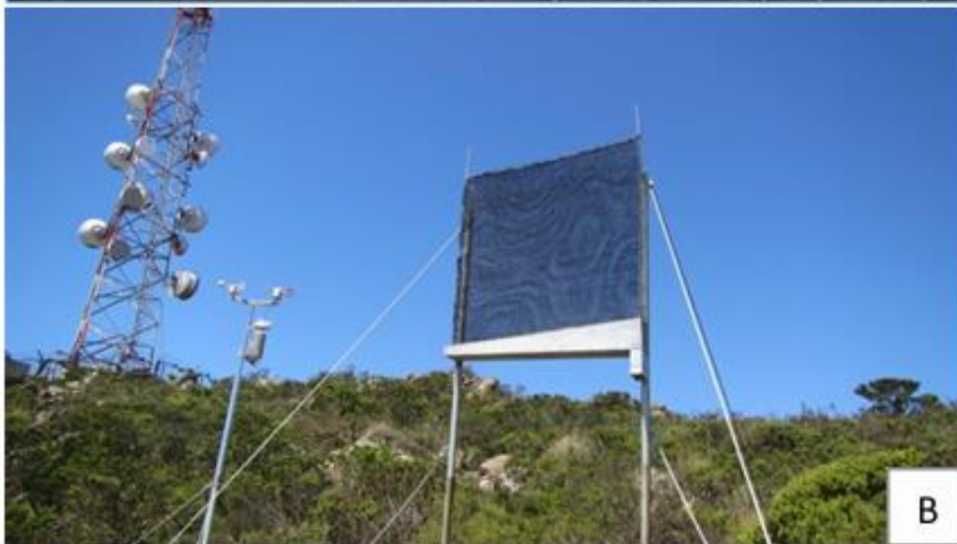
fog meter for water collection
