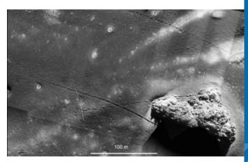
**Figure 8:** Imagery from Synthetic Aperture Sonar, showing a coral mound (lower right) and numerous trawl marks (curved and straight linear features). Data courtesy of Lundin Norway and the Norwegian Defence Research Establishment.
