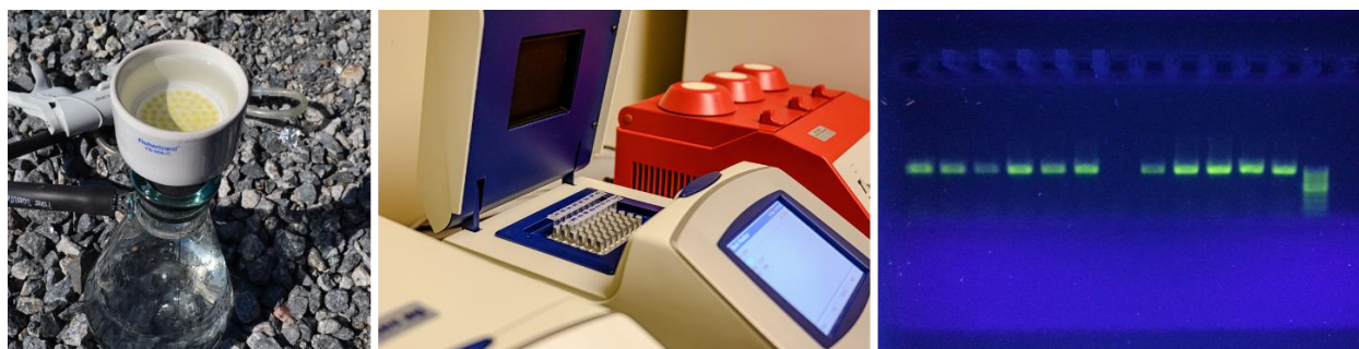
Figure 3. Researchers can collect environmental DNA in nature; PCR amplification with species-specific DNA primers can determine the species present in a water sample. Photos courtesy of (left to right) environmental DNA filtration apparatus by Katie Millette © 2021; PCR machine in the molecular genetics laboratory of the Conservatory and Botanical Garden of Geneva Switzerland, CJBG © 2021; gel electrophoresis image of amplified DNA fragments by Katie Millette © 2021.
