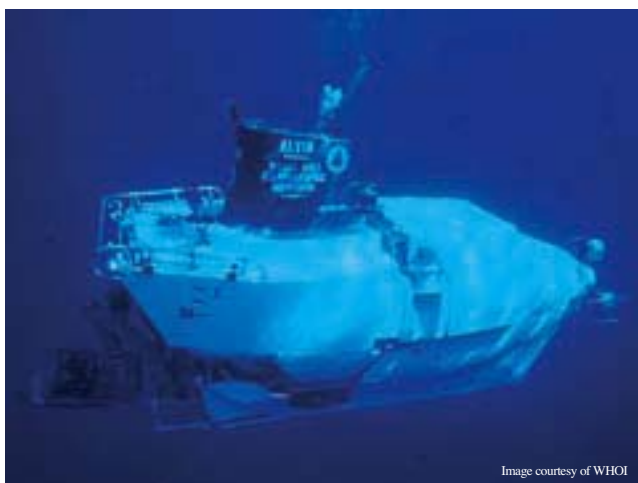
Alvin (pictured) has made over 4000 dives since it was built in 1964. The US Navy-owned submersible is operated by the Woods Hole Oceanographic Institution. A typical eight-hour dive takes two scientists and a pilot as deep as 4500 m. When working at maximum depth, it takes about two hours for the submersible to reach the seabed and another two to return to the surface. Alvin can hover, manoeuvre in rugged topography or rest on the bottom. Alvin’s most famous exploits include locating a hydrogen bomb accidentally dropped into the Mediterranean Sea in 1966, exploring deep-sea hydrothermal vents discovered two decades ago and surveying the sunken ocean liner Titanic
