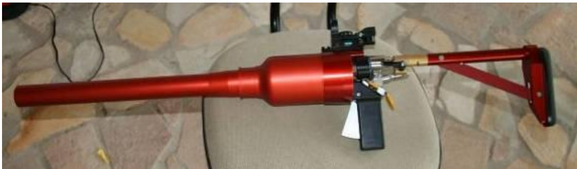
Fig. 2b – Gun ARTS used to deploy implantable tags.
