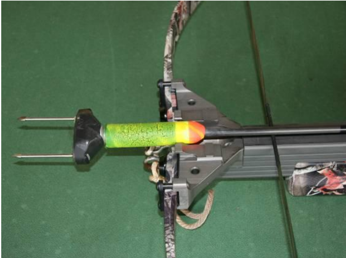
Fig. 1b - LIMPET tag with deployment arrow.
