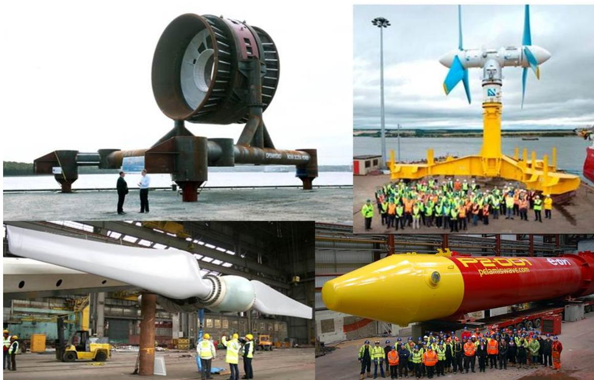
**Figure 1.** Examples of three leading tidal-stream turbines and one wave device. People in the pictures provide scale. Top left: OpenHydro ([www.openhydro.com](http://www.openhydro.com)), top right: Atlantis AK-1000 ([www.atlantisresourcescorporation.com](http://www.atlantisresourcescorporation.com)), bottom left: MCT SeaGen ([www.seageneration.co.uk](http://www.seageneration.co.uk)), bottom right: Pelamis Wave Power ([www.pelamiswave.com](http://www.pelamiswave.com)).
