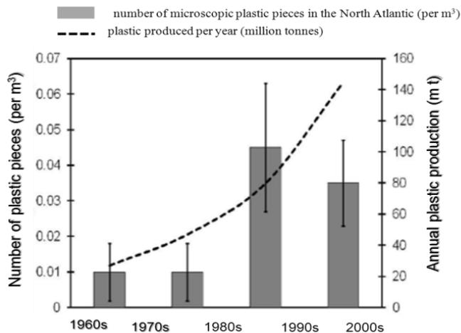
**Fig. 11. Microscopic plastics (< 5 mm) in surface waters, collected with continuous plankton recorder and identified by FT-IR, revealed a significant increase in abundance when samples from the 1960s and 1970s were compared with the 1980s and 1990s ( $F_{3,3} = 14.42$ ,  $p < 0.05$ ) (modified after Thompson et al., 2004).**
