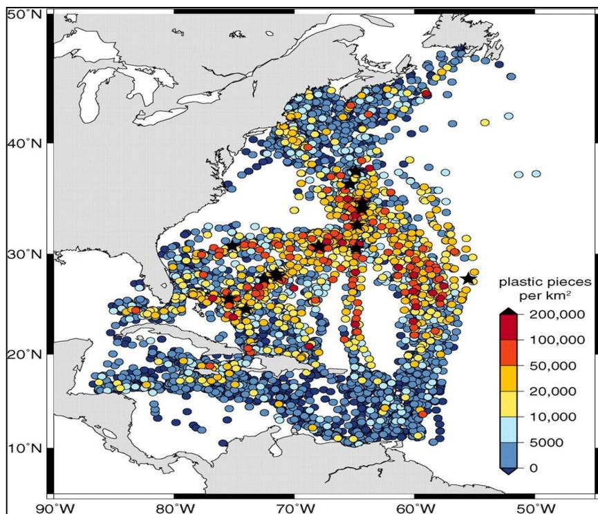
**Fig. 9.** Distribution of plastic marine litter collected in 6136 surface plankton net tows (1.0 x 0.5 m mouth with a 335  $\mu\text{m}$  mesh net) on annually repeated cruise tracks from 1986 to 2008 in the western North Atlantic Ocean and Caribbean Sea. Black stars indicate tows with measured concentration greater than 200,000 pieces per  $\text{km}^2$  (Law et al. 2010).
