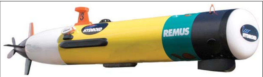
Figure 3.1. Autonomous underwater vehicle (AUV). Credit: Kongsberg Maritime.
