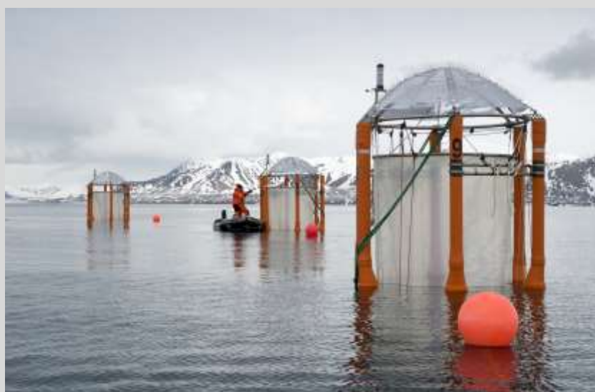
Experimental ocean acidification mesocosms in Svalbard, Norway. Photo: Maike Nicolai, GEOMAR. Seek permission
