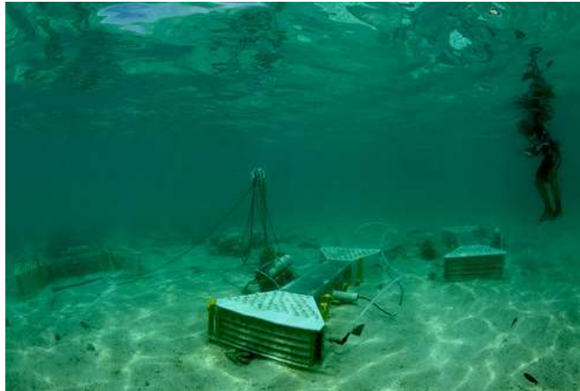
Figure 6.1. The coral proto-free ocean carbon enrichment system (CP-FOCE) deployed on Heron Island, Great Barrier Reef, Australia. Source: David Kline, Scripps. Seek Permission.
