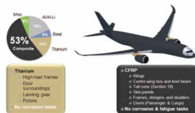
Figure 2: Airbus A350 XWB Airframe Use of Composites.
